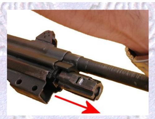
Now, we'll turn the bolt assembly facing forwards, insert it into the barrel assembly ...
