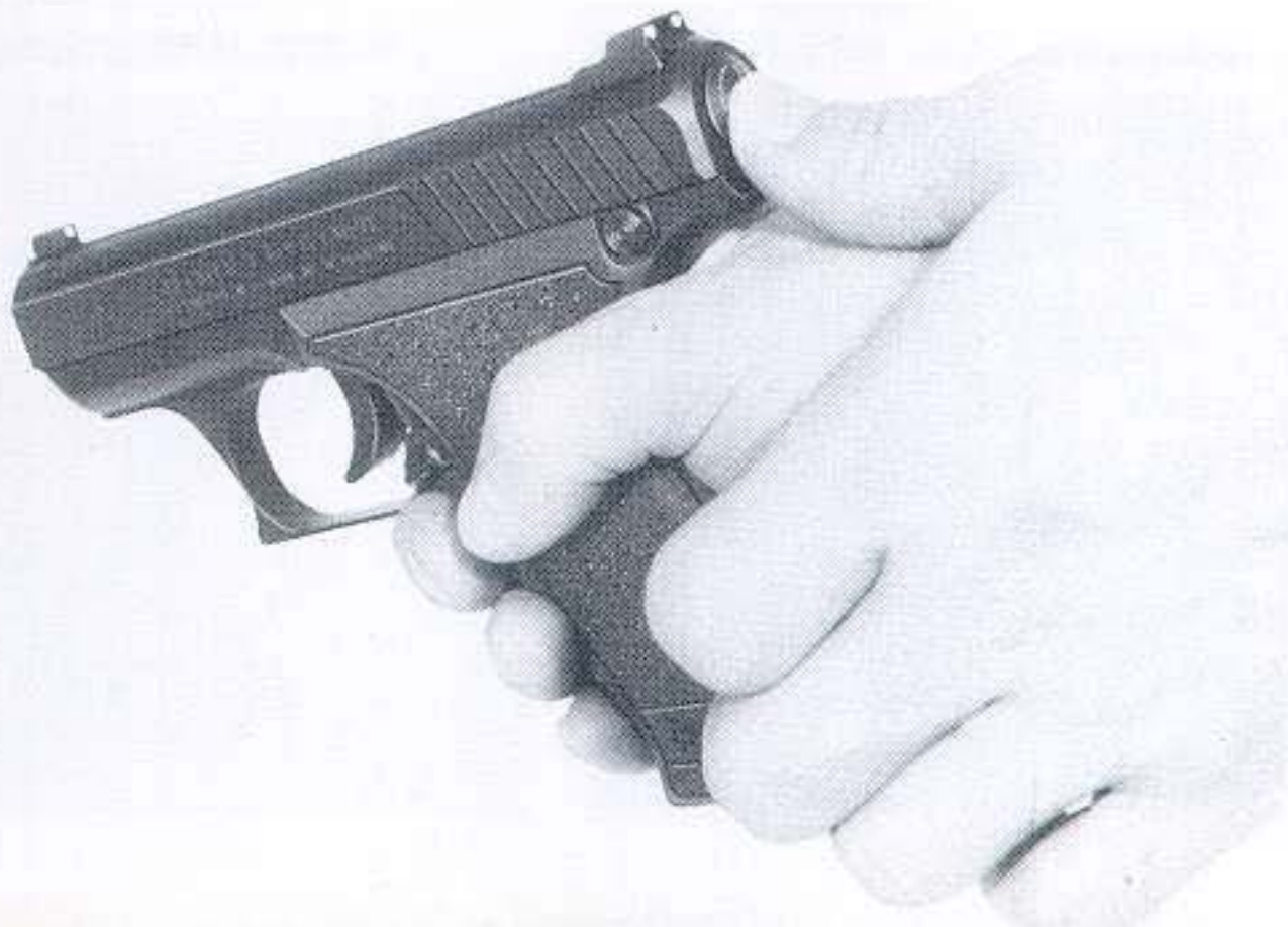
▼ Fig. 17: Press firing pin bushing forward
