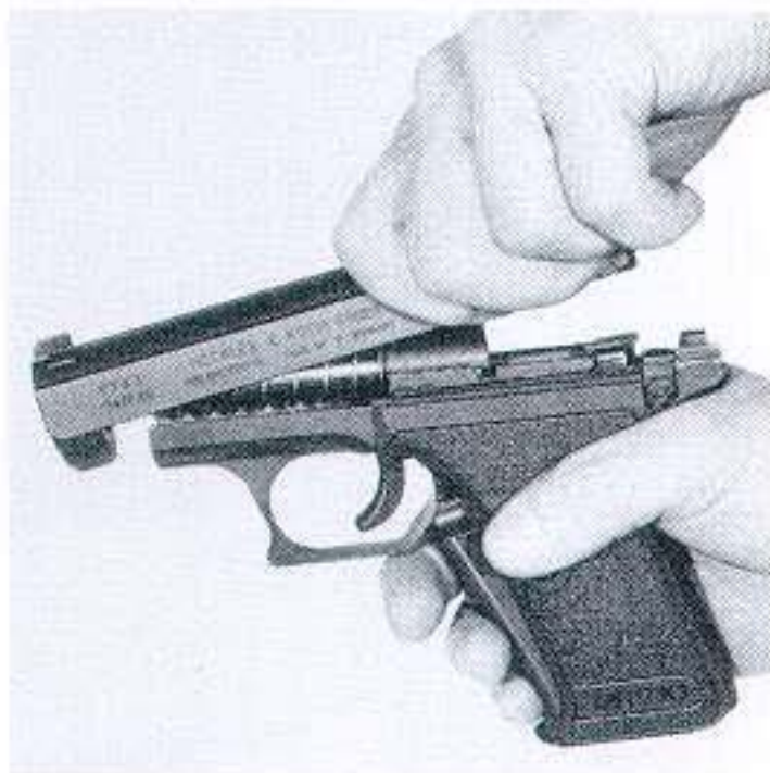
Fig. 9: Place slide on receiver
