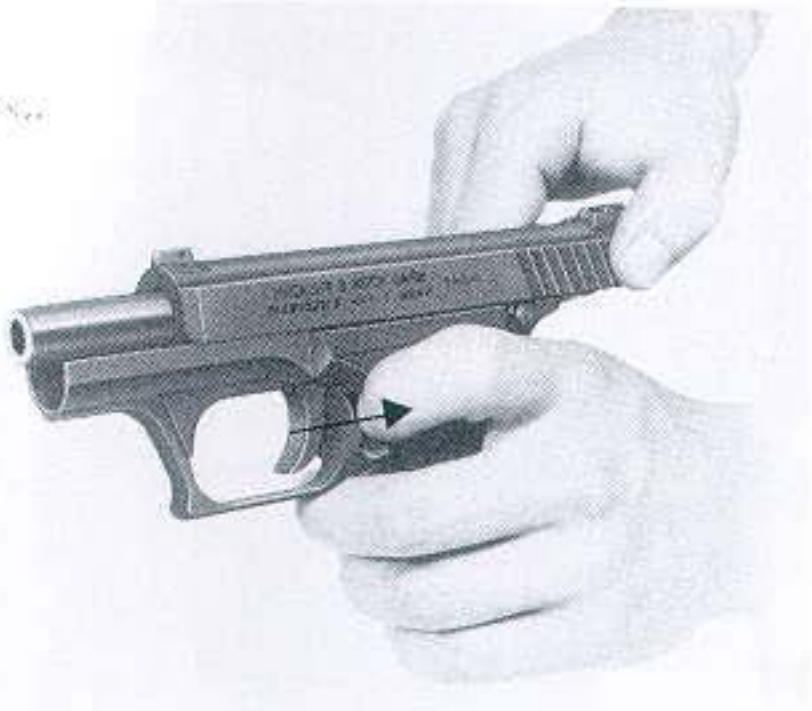
Fig. 6: Press in slide catch lever
