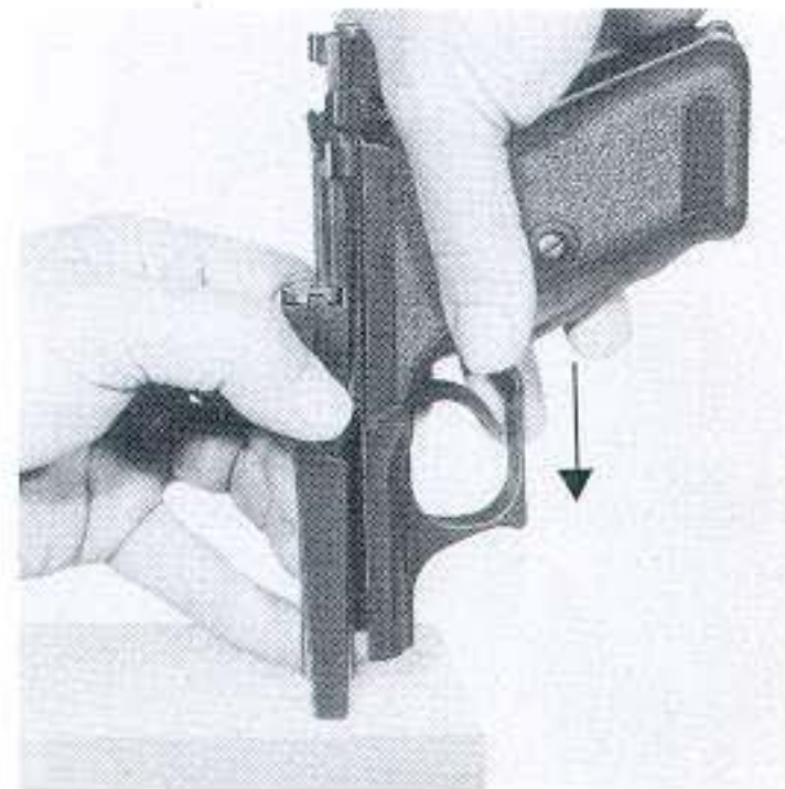
Fig. 13: Loosening the chamber
